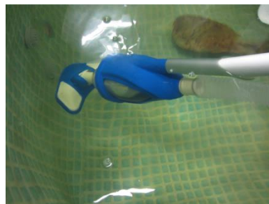
Connect vacuum hose and vacuum head under water
