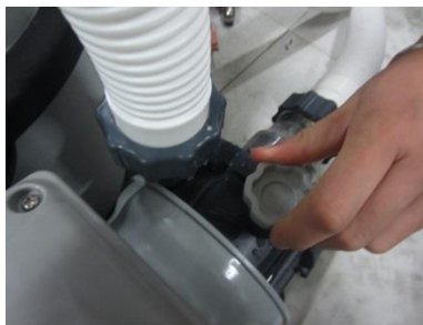
Release air from sand filter pump
