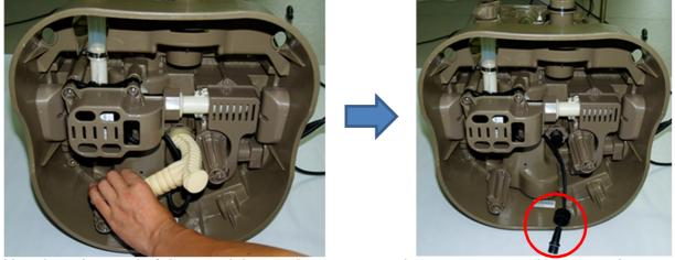
3) Use the other end of the special wrench to unscrew the motor connection nut and remove the motor cover using a Philip screw driver:
