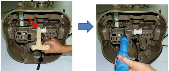
4) Pull the filter motor out:
