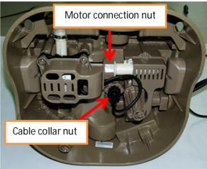
2) Use the <u>special wrench tool that is included</u> with replacement filter motor to unscrew the motor cable collar nut. Pull the motor cable out:
