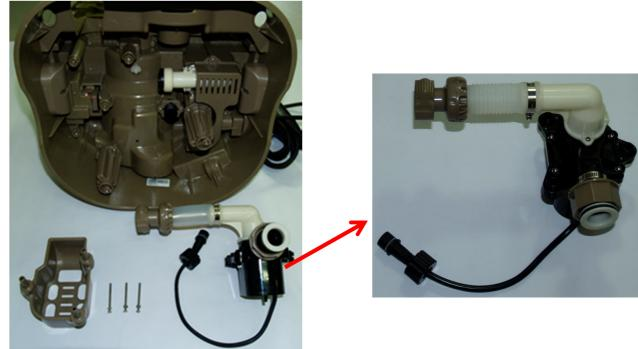
5) Install the new filter motor back by reversing the above steps.
