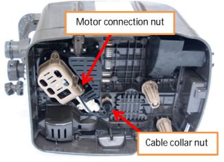
2) Use the **special wrench tool that is included** with replacement filter motor to unscrew the motor cable collar nut. Pull the motor cable out:
