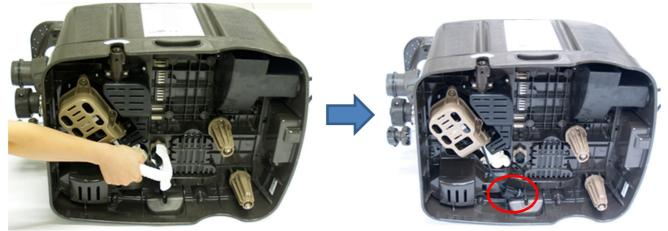
3) Use the other end of the special wrench to unscrew the motor connection nut and remove the motor cover using a Philip screw driver:
