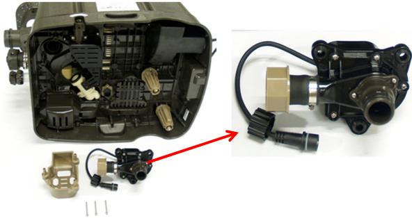
5) Install the new filter motor back by reversing the above steps.
