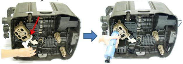
4) Pull the filter motor out:
