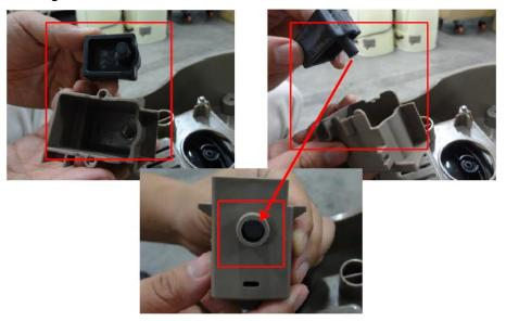
7. Reverse steps 2,3 and 4 to reconnect the thermal protector. Firmly press the "RESET" button on the side of the control base using a suitable long and rigid object till the E98 alarm stop.
