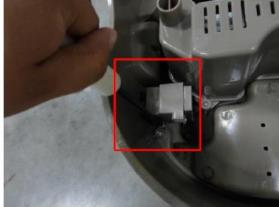
3. Pull out the reset button box and unscrew the two screws on the bottom of the box.
