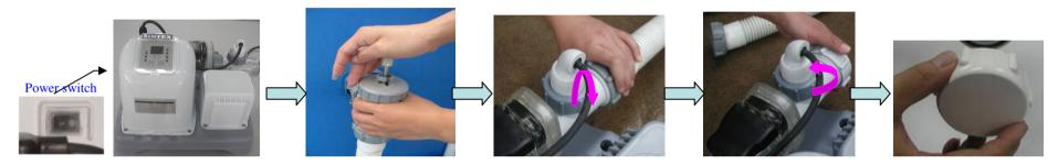
**STEP 2:** Disassemble the nut and lift up the copper electrodes.
